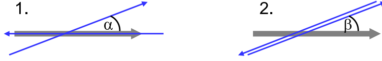
Figure 6.15. An alignment of the laser and the ion beams. In the first case was one of the laser beams properly overlapped with the ion beam and the other laser beam was slightly misaligned. The second test was with two laser beams properly overlapped but they were slightly misaligned relative to the ion beam.
