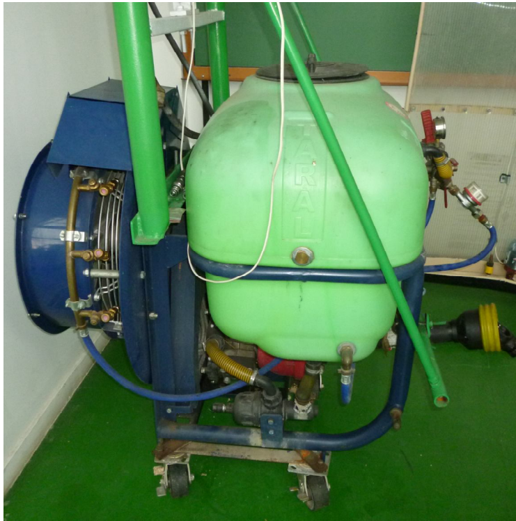
Figure 1. Sprayer for pest and disease control in vineyards and intensive orchards, type TARAL 200 PITON TURBO
