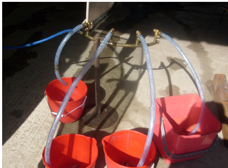
Figure 2. Collection of solution sprayed from each nozzle to spray machine type TARAL 200 PITON TURBO
