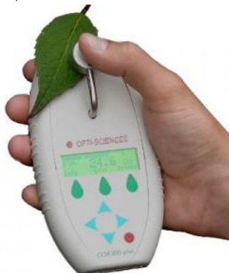
Figure 3 Device for determining the chlorophyll content of leaves ( http://www.envcoglobal.com )
