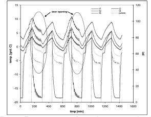
Figure 4 Energy consumption and temperature levels (10% load; with door opening;  $25^{\circ}$ C)
