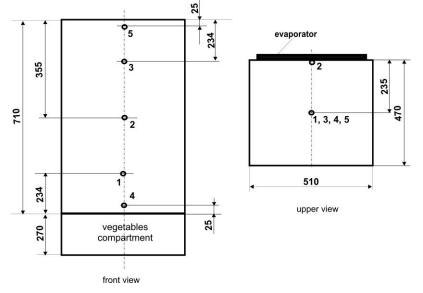
Figure 1 **Placement of the temperature probes** 1, 3, 4 – temperature probes according to EN 15505:2005; 2, 5-additional temperature probes.
