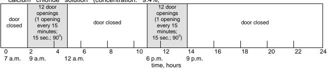
Figure 3 Test program with refrigerator door opening
