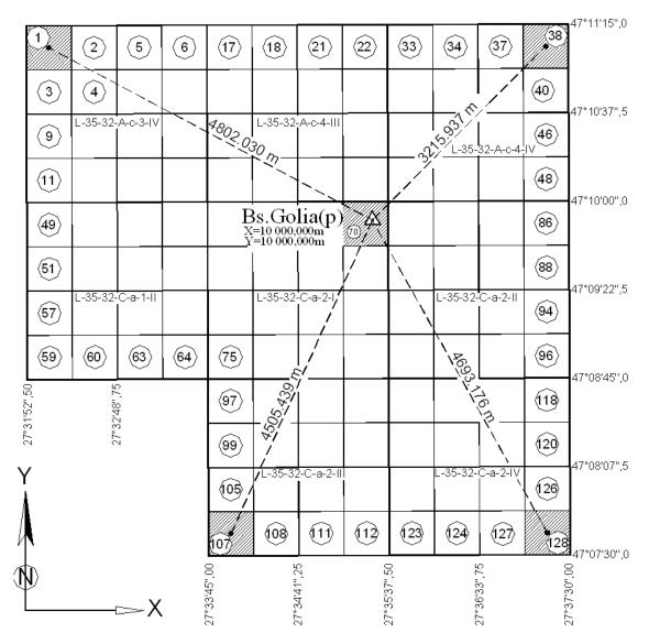
Figure 2 Cartographic base of geodetic trapeziums, scale 1:5 000
