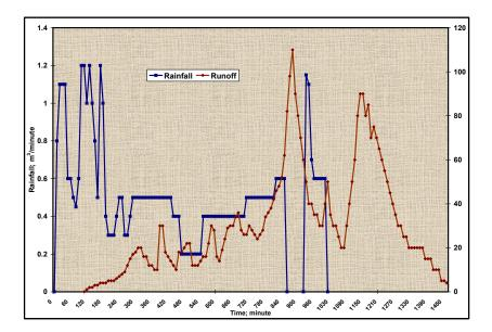
Figure 5 - Runoff (I/minute) hydrograph, on September 7, 1989, in Scobâlțeni watershed
