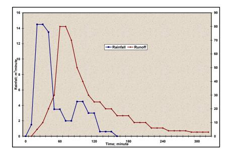
Figure 7 - Runoff (I/minute) hydrograph, on April 24, 2008 , in Scobâlțeni watershed
