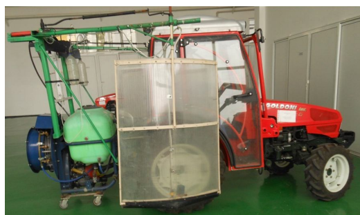
Figure 2 Vineyard spraying equipment a) work position; b) transport position.
