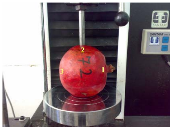
Figure 1 - Locations on the fruit where mechanical properties were measured by penetration probe
