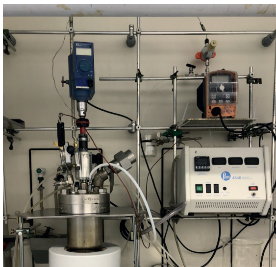
Figure 4.15. Reaction set-up for hydrolysis of polyester experiments.
