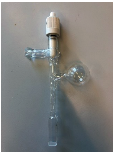
Figure 5.10. J. Young type UV-Vis cuvette with additional mixing volume.
