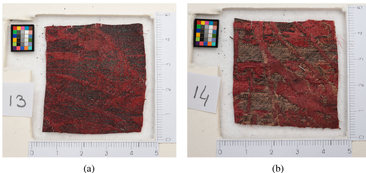
Fig. 4 (a) Sample 13 (40×40mm), corroded silver threads (black), largely unravelled; (b) sample 14, corroded silver threads (black), mostly intact together with the silk thread that forms their core (brown).
