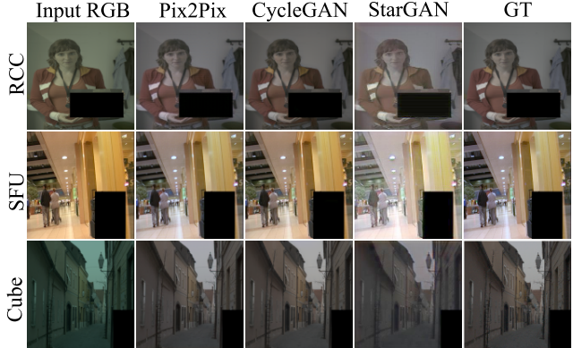
Figure 3. Performance of different GAN models on the color constancy task. All models can recover proper white balanced images. The images are gamma adjusted for visualization.
