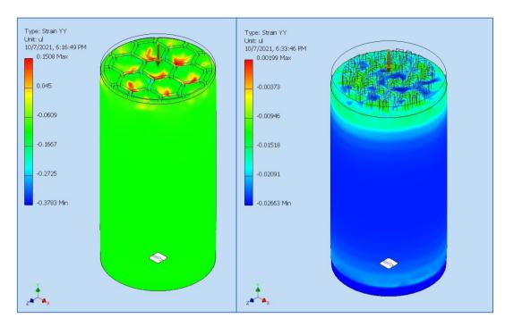
Fig. 5 - Compressive strain result for samples 3 (left) and 8 (right)
