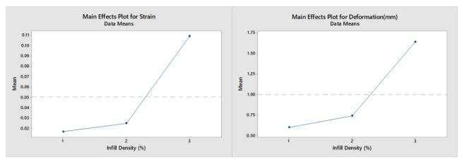
Fig. 7 - Main effect plot of infill density (%)
