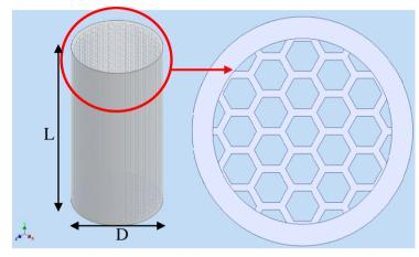
Fig. 3 - Internal hexagonal structure design
