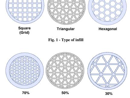
Fig. 2 - Different infill density structures for the sample
