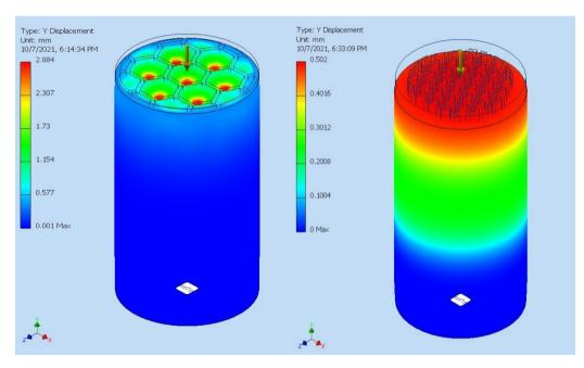
Fig. 6 - Total deformation result for samples 3 (left) and 8 (right)
