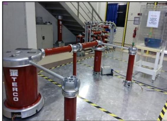
Fig. 2 - The HVDC breakdown test setup
