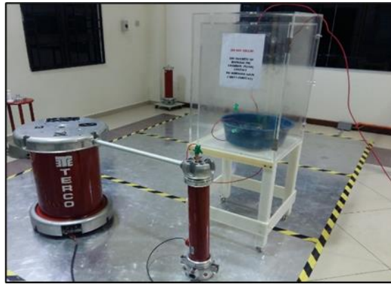
Fig. 1 - The HVAC breakdown test setup
