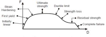
Fig. 1 - Concrete material nonlinearity
