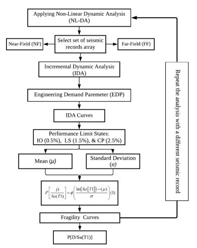
Fig. 5 - General steps for the development of the fragility curves
