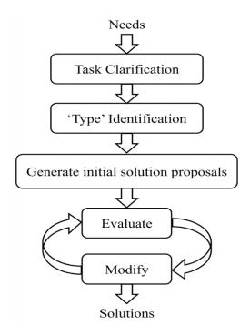
Figure 7. Proposed 'prescriptive' design synthesis process.
