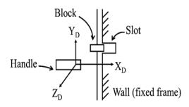
Figure 2. The components of a simple door latch where, the coordinate system  $(X_D, Y_D, Z_D)$  is attached to the door.
