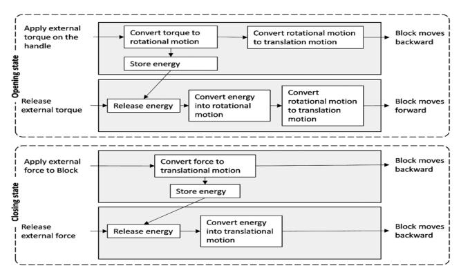
Figure 3. Function diagram of a multi-state door-latch system.
