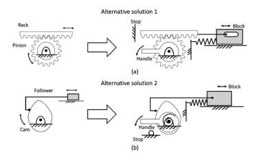
Figure 11. Two more alternative solutions are generated with support from the tool.
