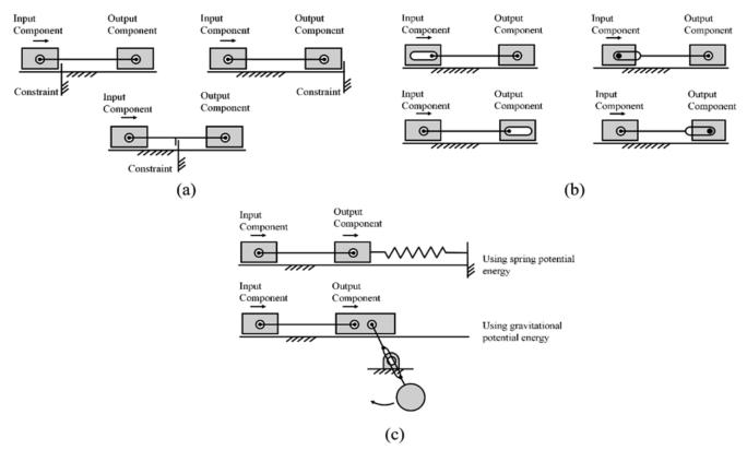
Figure 10. The modification rules are demonstrated through examples: (a) Different ways of imposing constraints, (b) Different ways of modifying interfaces and (c) Different ways of adding an artificial effort.
