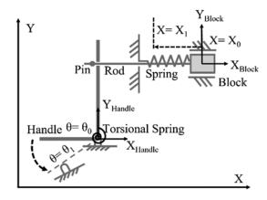
Figure 5. Schematic representation of the door latch.
