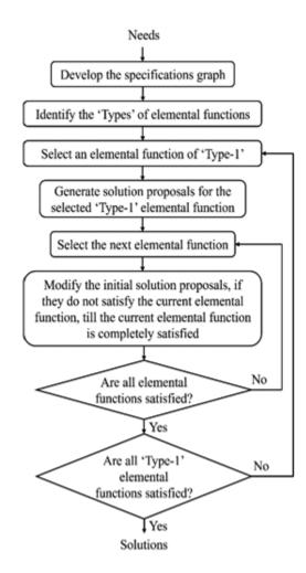
Figure 9. Detailed steps in the prescriptive design process.
