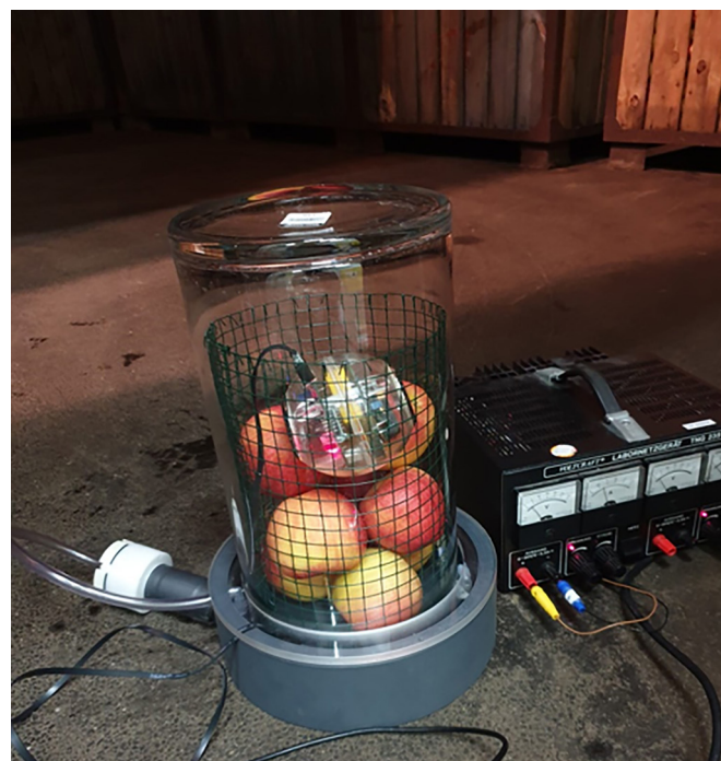
Figure 6. Modular sensor system RMS88 and respirometer installed in a commercial storage facility of apples to measure in-situ real-time respiration rate and RQ.
