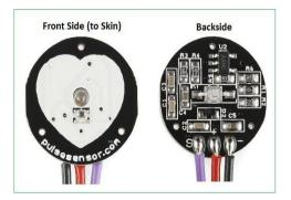
Figure 2. Pulse Sensor
