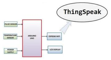
Figure 1. Proposed Prototype Block Diagram[6]
