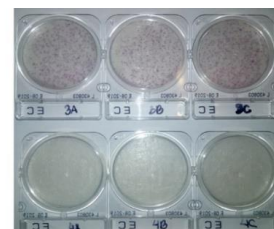
Fig. 3. Water testing kits indicate results of contaminated (upper level) and cleaned water (lower level)
