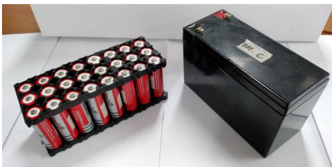
Fig. 4. Lithium-ion battery system and Lead-acid motorcycle battery
