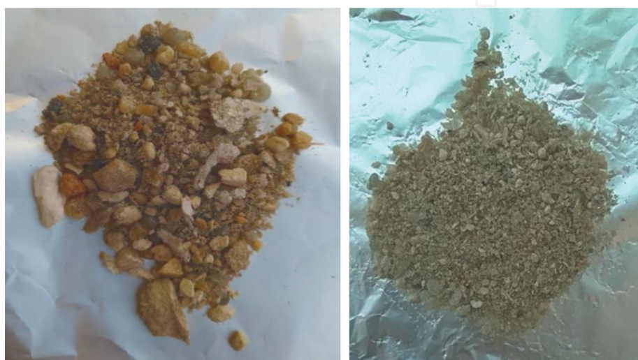
Figure 10. EPS sample before (left) and after (right) shredding for TGA analysis.
