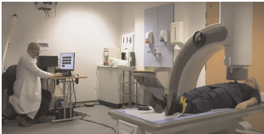
Figure 3. 9-channel MCG-system (Cardiomox) in unshielded hospital setting.
