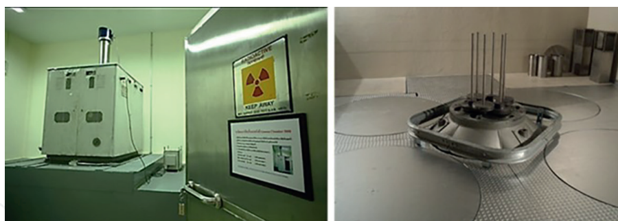
Figure 1. (left) Gammator and (right) Gamma room at Thailand Institute of Nuclear Technology (Public Organization).
