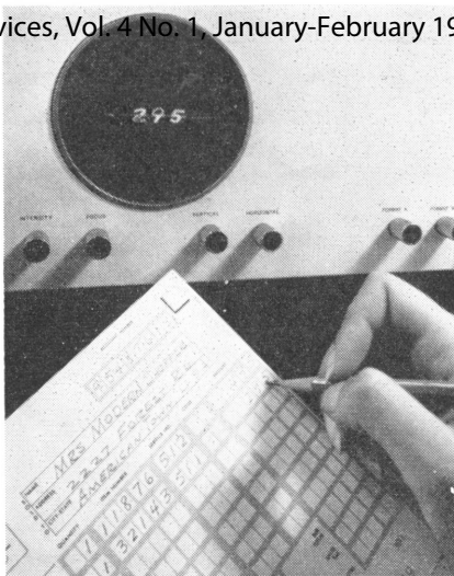
Scope of 1287 reader reproduces image of handwriting on sales check.
