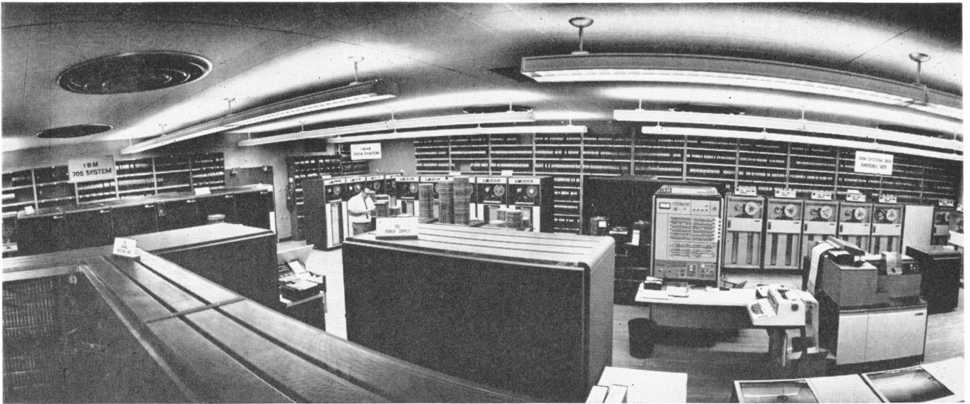
In a rare display of almost the entire history of computers, this data processing room at Aetna Life & Casualty Insurance, Hartford, Conn., houses three generations of computers all of which are still in use. At left is IBM 705, which uses vacuum tube circuits; in center is IBM 7074, which uses transistorized circuits; at right is IBM System/360 Model 365 with micro-miniaturized circuits. A job that took the 705 four minutes takes six-tenths of a second on the 360.
