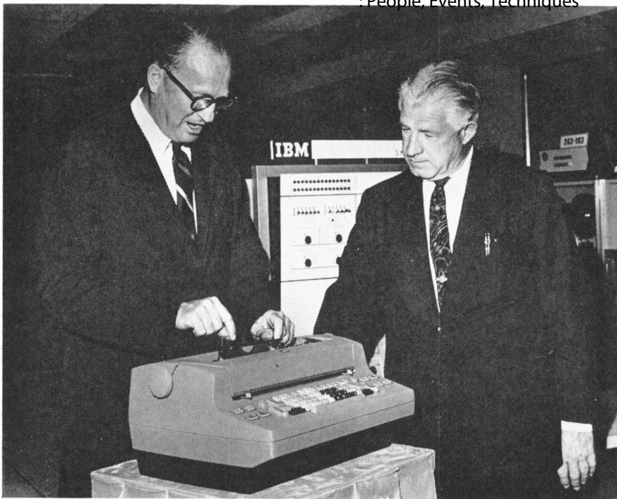
Terminal device, designed by IBM for Household Finance Corporation, will transmit information from branch offices all over country to headquarters in Chicago.
