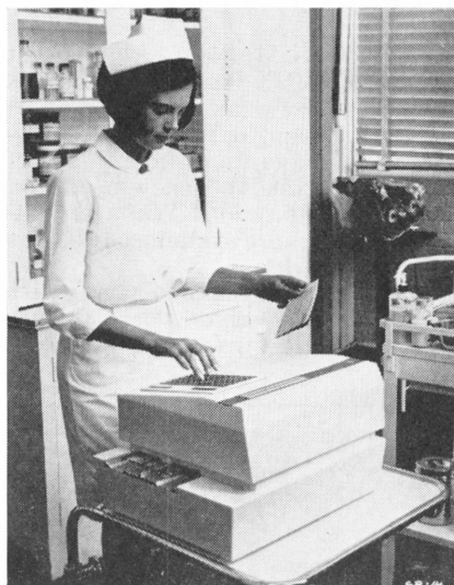
The Standard Register Company's new source record punch will record information in both human-readable language and machine-readable code on the same document at the same time in a single operation.
