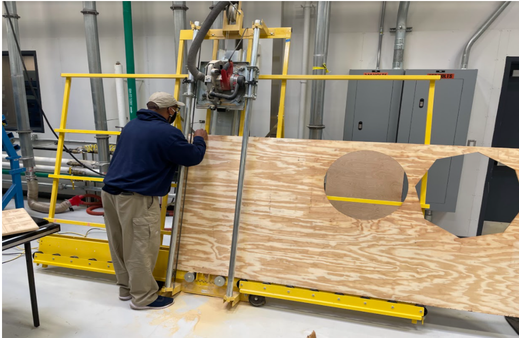
Figure 10. Vertical Band Saw for Wall Slab Cutting
