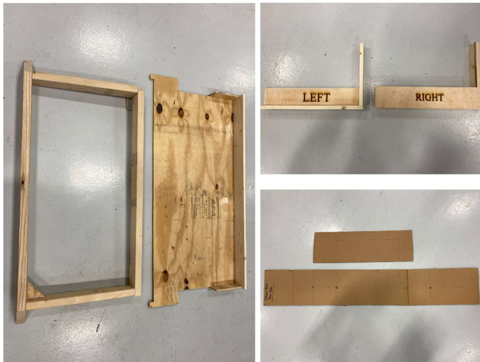
Figure 6: Poke Yokes used in the building process.
