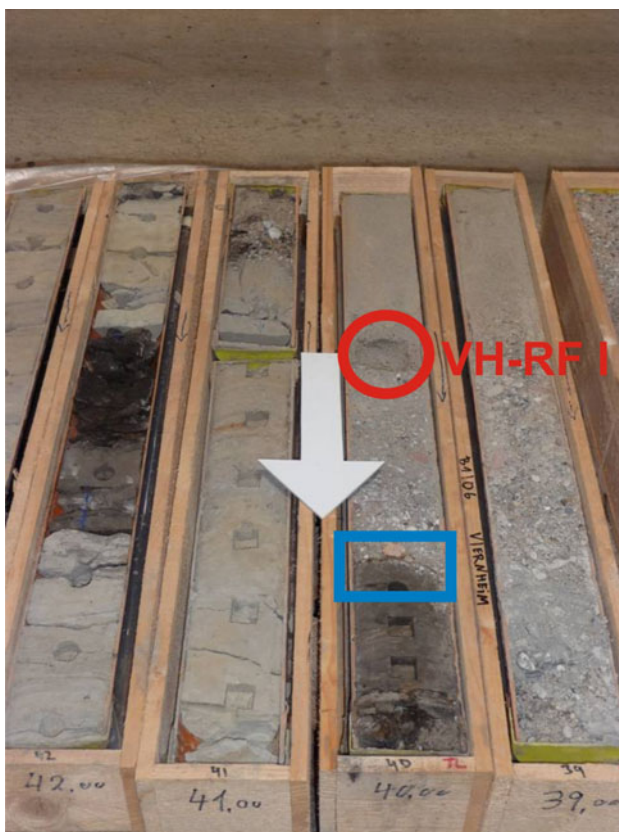
Fig. 4. This photograph shows the core sections of the Viernheim core from 39 m – 42 m core depth. This core part represents the transition (marked by the bin) from the coarse-grained and gravel rich upper fluvial units and the Upper Interlayer which is characterized by finer material and a high content of organic material. Sample VH-RF I was taken directly on top of the Upper Interlayer as marked by the circle.
