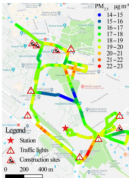
Figure 12. Overall spatial distribution of PM 2.5 along the fixed route during the CARE campaign. Map data © Google Maps 2015.
