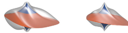
Figure 9: Uncertainty glyph using superquadric (left) and the glyph from Gerrits et al. [GRT17] (right) as base for an indefinite mean tensor (image from [GRT19]).
