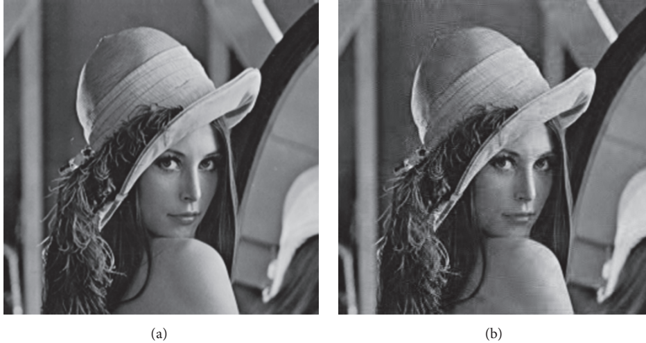
FIGURE 4: STP-CS for image. (a) is the original image. (b) is the recovery image. The measurement matrix is a Gaussian matrix, and the recovery algorithm is OMP.
