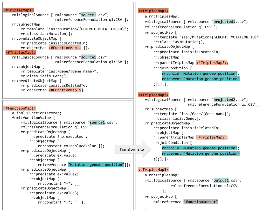
Fig. 3: Example of DTR and Object-based MTR. On the left, an exemplary mapping including two TriplesMaps and a FunctionMap provided by the original data integration system. On the right side, the mappings are transformed by FunMap including two new TriplesMaps and one new TriplesMap.
