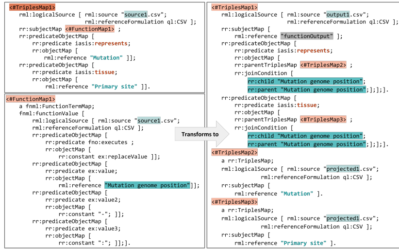
Fig. 6: Example of Subject-based MTR. An example of mappings including a TriplesMaps and FunctionMap are illustrated on the left and their transformed version including three TriplesMap are shown on the right side.
