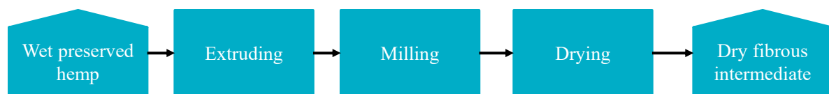
Figure 5. Main steps for the processing of wet preserved hemp raw materials in the Leibniz Institute for Agricultural Engineering and Bioeconomy (ATB) pilot plant.
