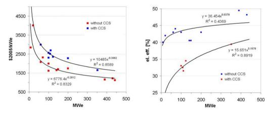
Figure 1: Techno-economic data of BIGCC processes with and without CCS obtained from the literature. Left: Specific investment costs (\$2005/kWe) vs. installed capacity (MWe). Right: Electrical efficiency vs. installed capacity (MWe).
