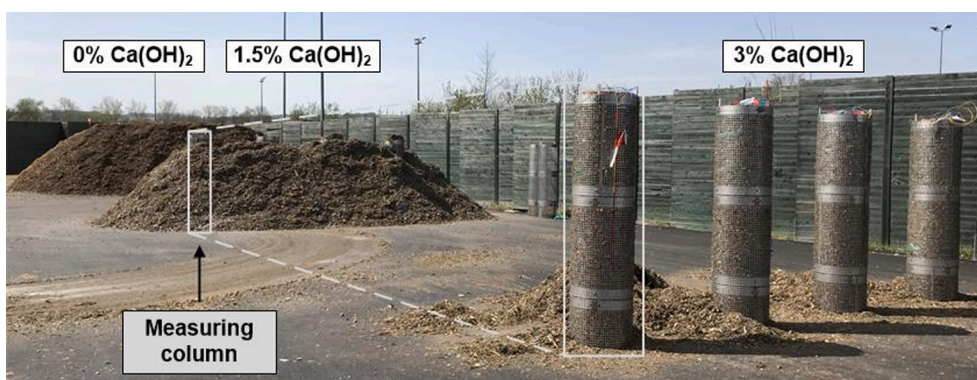
Fig. 1. Construction of the wood chip piles and installation of the measuring columns.
