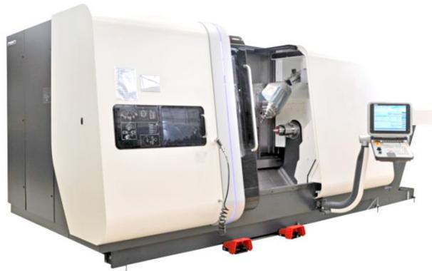
Fig. 3. Universal lathe DMG MORI CTX gamma 1250 TC [IWF].
