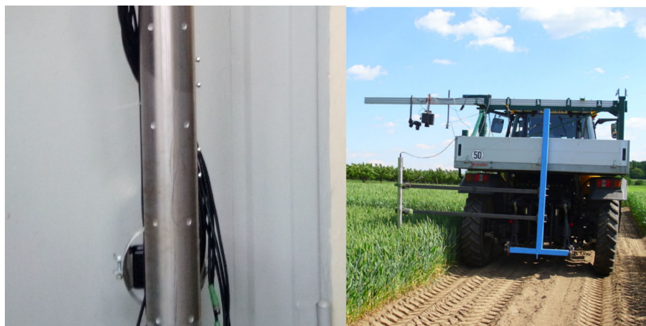
Figure 1. Section of the middle in-canopy sensor tube (left) and attachment to the rear of the tractor using a three-point linkage on a movable device during measurements in the plots (right).
