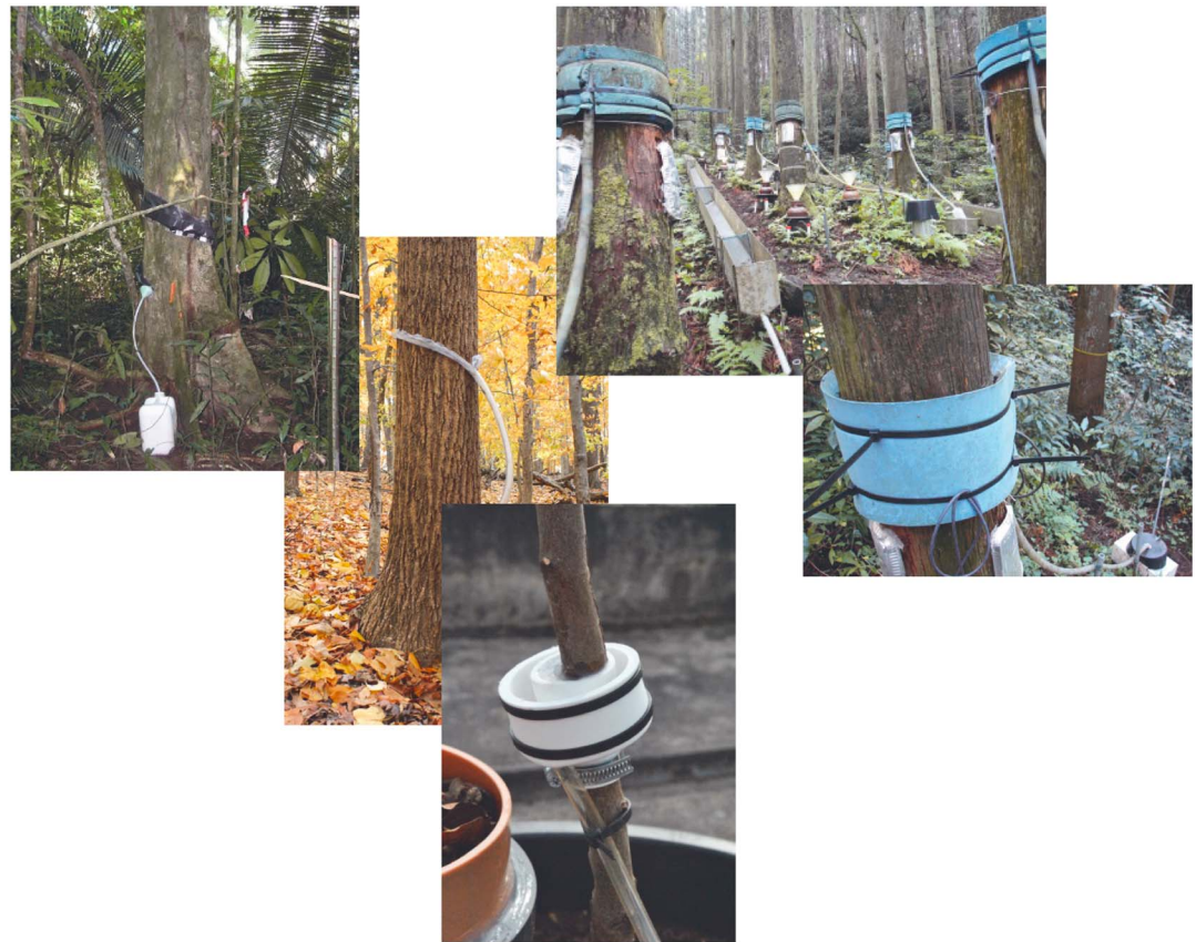
Figure 3. Examples of stemflow collectors as used by (top left) Germer et al. [2010] in Rondônia, Brazil, (middle left) Levia et al. [2010] in northeastern USA (photo courtesy N. Finger), (bottom left) Levia et al. [2015] for saplings in Thuringia, Germany, and (top right and bottom right) Iida et al. [2012] in Tsukuba Experimental Forest, Japan (photos courtesy K. Nanko and S. Iida).
