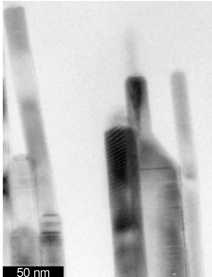
Figure 4.17: TEM image of NW tips of sample A0c . The density of the SFs identified by the horizontal black striation is largely reduced compared to sample A0a in Figure 4.6.
