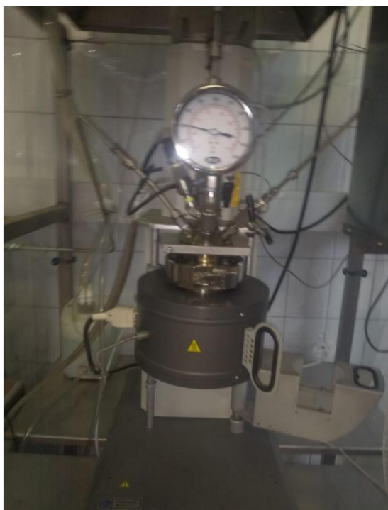
Figure 4. Pilot-scale stirred tank stainless steel reactor of 1.0 L (Parr, Moline, IL, USA, Model: 4577).
