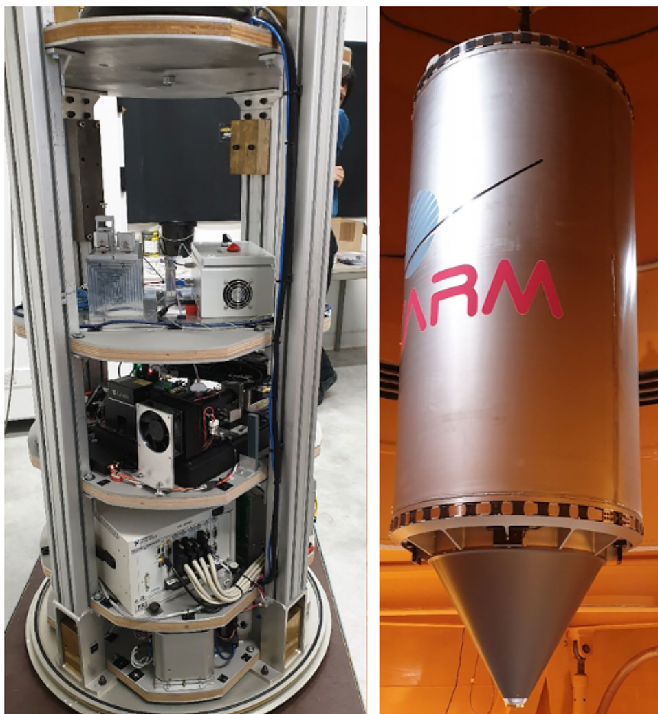
Fig. 10 Photograph of the dynamic light scattering instrument and the liquid handling set-up inside the open drop tower capsule (left) and of the sealed capsule (right)
