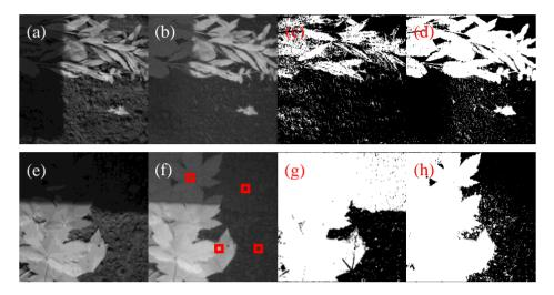
For the shadow soil region the NDVI is overrepresented and for the reNDVI $_{CMOS}$  a threshold of 0.1 is almost reasonable. Applying the range-extended NDVI $_{CMOS}$  algorithm to the image in Figure 10(c) generated the result shown in Figure 13.
