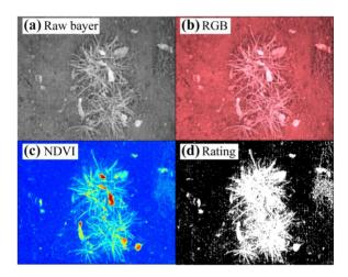
Figure 10. (a) Raw image of tufts of grass and leafs added by wind, (b) false color image, (c) NDVI image in rainbow colors from blue (zero) to red (256), and (d) binary image under direct angular sunlight and a shutter time of 90 μs.
