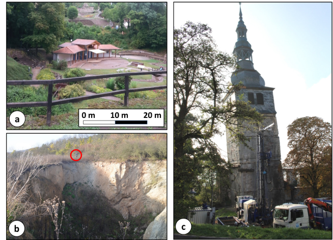
Figure 3. Subrosion signatures at the surface in Bad Frankenhausen and the surrounding area. (a) The oldest sinkhole of the region, called “Quellgrund”, is located in the medieval city center of Bad Frankenhausen and used today as recreation area. (b) One of the most recent sinkholes is found directly beside the “Äbtissinnen Grube” (red circle marks a person standing at the sinkhole margin). (c) The most famous subrosion phenomenon is the leaning church tower of Bad Frankenhausen (height of 56 m); note borehole in foreground.
