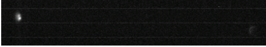
FIGURE 7: The combined image of \approx 1200 guiding frames on 51 Peg, total exposure time 20 minutes. The bright image to the left is the position of the star as imaged through the beam splitter the fainter image to the right is the light spilled over the fiber entrance and reflected back onto the guider camera. Guiding is done exclusively at the brighter image. Aperture photometry of the combined frame is used to measure the amount of light lost, here 32%.
