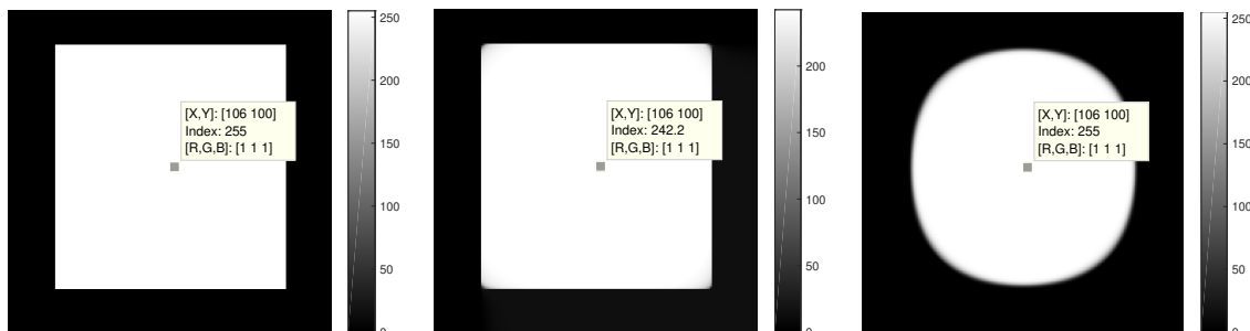
Figure 1: An example that distinguishes the damped second-order MCF and the damped second-order TVF. From left to right: the square image; the result of damped second-order TVF (middle) and the result of damped second-order MCF (right).
