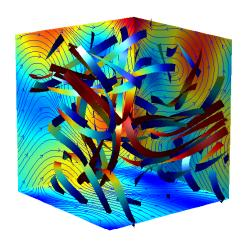
Figure 1: The velocity solution to the Ethier-Steinman problem with a=1.25, d=1 at t=0 on the  $(-1,1)^3$  domain. The complex flow structure is seen in the streamribbons in the box and the velocity streamlines and speed contours on the sides.
