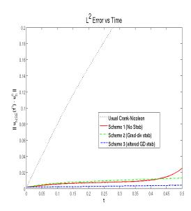
Figure 2: The plot above shows  $L_2$  error of the velocity vs time for the four schemes of test 2. We see in the plot that the stabilizations add accuracy to the enhanced-physics scheme, and that the altered grad-div stabilization gives slightly better results than the usual grad-div stabilization. It can also be seen that the enhanced-physics scheme is far more accurate in this metric than the usual Crank-Nicolson scheme.
