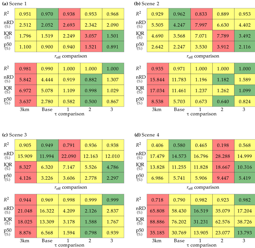
Figure 8. (a) Comparison of retrieved cloud optical thickness ( \tau , c, d) and effective droplet radius ( r_{\text{eff}} , a, b) from the native LRES (at a scale of \approx 3 km) and baseline retrievals (i.e., only accounting for low-resolution reflectance variability), as well as the downscaling experiments 1 (statistical downscaling approach), 2 (constant reflectance ratio approach), and 3 (adjusted lookup table approach with LUT slope adjustment), and the reference retrieval results. Parameters to quantify the comparisons are the median of the relative difference to the reference (p50), relative interquartile range (IQR; 75th–25th percentile of the relative difference to the reference), normalized root-mean-square deviation (nRD; defined as the RD between the two data sets, normalized by the average reference retrieval), and the explained variance ( R^2 ). Green colors indicate the experiment that compares best to the reference results, i.e., highest R^2 and lowest p50, IQR, and nRD. Red colors indicate the experiment with the worst agreement with the reference retrievals, while yellow colors indicate all experiments in between. Data are from example scene 1 sampled on 1 June 2013 at 10:05 UTC. (b)–(d) Same as (a) but for example scene 2 to 4, respectively.
