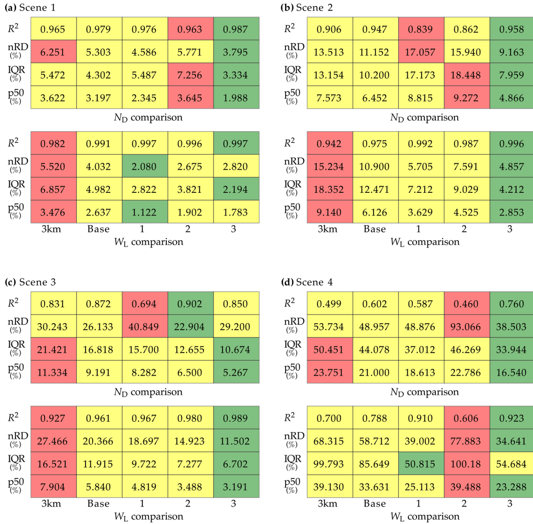
Figure 10. (a) Comparison of derived liquid water path ( W_L , c, d) and droplet number concentration ( N_D , a, b) from the native LRES (at a scale of \approx 3 km) and baseline retrievals, as well as the downscaling experiments 1 (statistical downscaling approach), 2 (constant reflectance ratio approach), and 3 (adjusted lookup table approach with LUT slope adjustment), and the respective reference results. Parameters to quantify the comparisons are the median of the relative difference to the reference (p50), relative interquartile range (IQR; 75th–25th percentile of the relative difference to the reference), normalized root-mean-square deviation (nRD; defined as the RD between the two data sets, normalized by the average reference retrieval), and the explained variance ( R^2 ). Green colors indicate the experiment that compares best to the reference results, i.e., highest R^2 and lowest p50, IQR, and nRD. Red colors indicate the experiment with the worst agreement with the reference retrievals, while yellow colors indicate all experiments in between. Data are from example scene 1 sampled on 1 June 2013 at 10:05 UTC. (b)–(d) Same as (a) but for example scenes 2 to 4, respectively.
