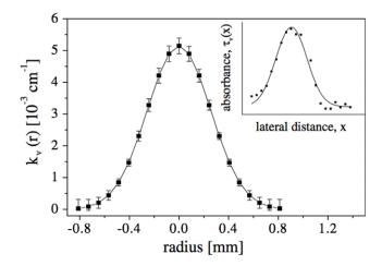
**Figure 17.** Radial profile of  $N_2(A)$  absorption coeficient obtained after Abel inversion of CRDS lateral absorbance measurements in a nitrogen nanosecond repetitively pulsed discharge. The inset shows the lateral absorbance distribution [18] (© IOP Publishing. Reproduced with permission. All rights reserved).
