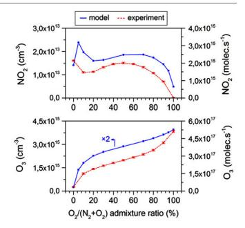
Figure 26. NO<sub>2</sub> and O<sub>3</sub> densities in a multipass measurement chamber obtained by QCLAS and calculated data from a RF-jet model in different  $O_2/(O_2 + N_2)$  ratios. From [267].
