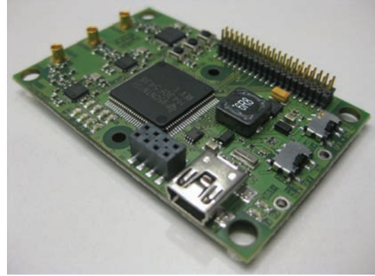
FIGURE 5: FeuerWhere Node of IHP, a wireless sensor node equipped with three radios, external flash memory and an ultralow power microcontroller.
