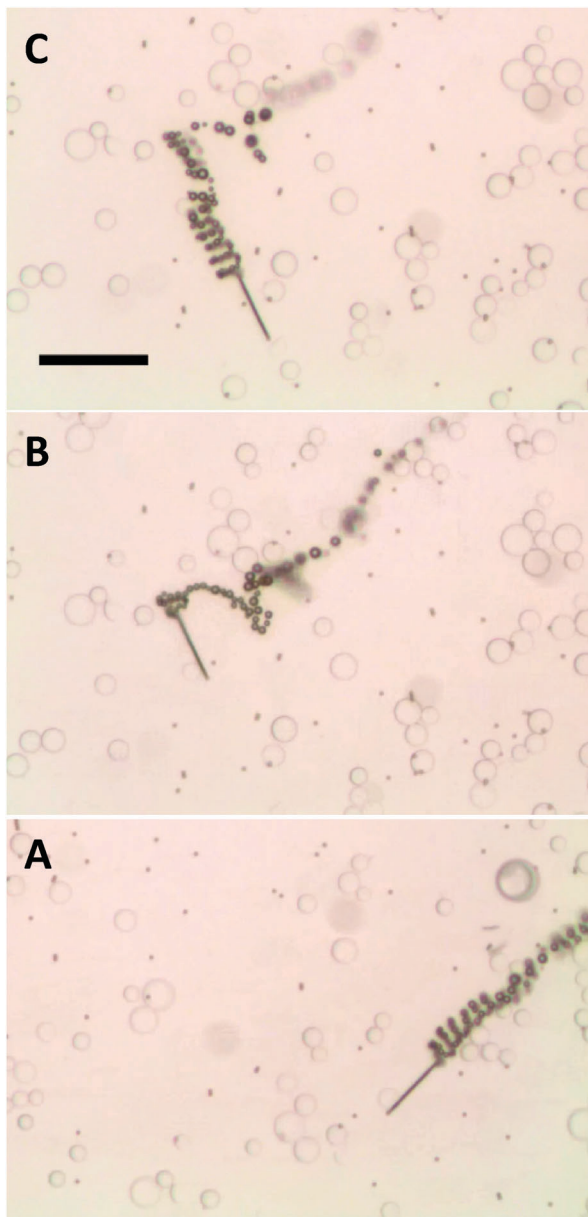
Fig. 3 Non-magnetized microjets are not capable of pick-up of paramagnetic beads (dark spots) from their mixture with silica beads (transparent beads), moving through their mixture and ignoring them all. A, B and C represent time 0, 3 and 5 s of time frame. Scale bar of 50 \mu\text{m} . Conditions: 6% \text{H}_2\text{O}_2 , 1% SDS, beads concentration approximates to 3 \times 10^4 \mu\text{L}^{-1} for the silica beads and 1 \times 10^4 \mu\text{L}^{-1} dynabeads.
