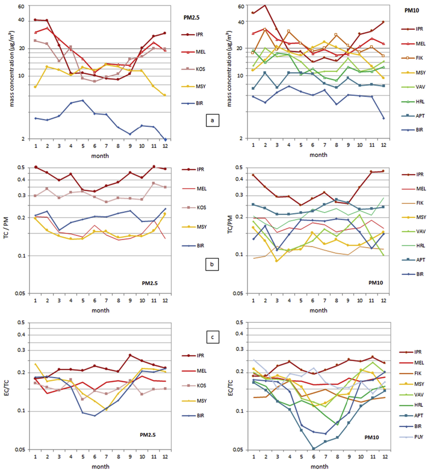
Fig. 12. Seasonal variations in (a) PM mass concentrations, (b) TC/PM and (c) EC/TC ratios. Lines without full symbols correspond to the sites for which sampling artefacts were not addressed (see text).
